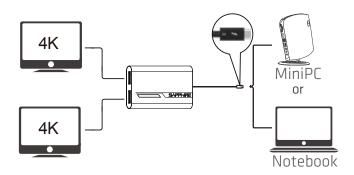
The DisplayPort dongle drives up to a single 5K resolution @60 Hz. (Windows only)
