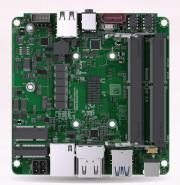
The SAPPHIRE BP2-FP5 4"x4" small form factor embedded motherboard is based on the latest AMD Ryzen™ Embedded V/R Series Family of APUs which feature the industry leading Vega GPU graphics combined with the quad/dual-core high-performance "Zen" CPU.
